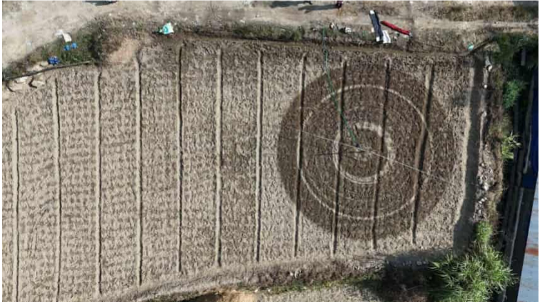
Figure 11 Drone image showing the irrigation pattern of the Smart Sprayer, with two dry circles corresponding to gaps in irrigation at the arm connections.
