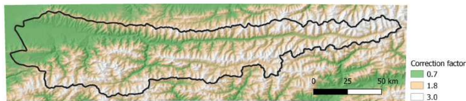
Figure 53. The Precipitation correction factor. The original downscaled ERA5-TopoSCALE precipitation data is divided by this elevation-dependent correction factor
