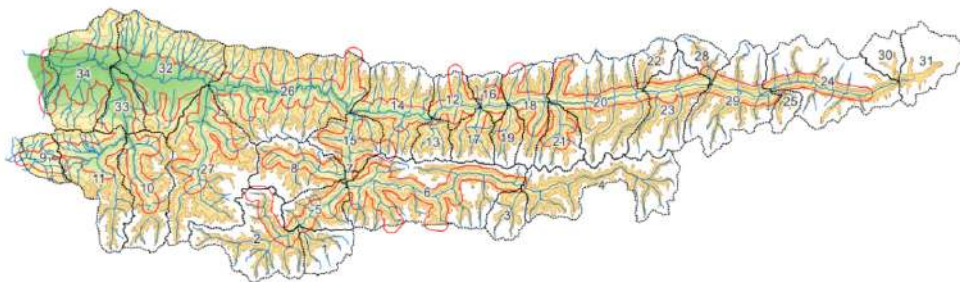
Figure 73. ZRB where red lines indicate 2-km buffers around the existing road network. The area in between the red lines is accessible by car. The color gradient in the background indicates elevation.
