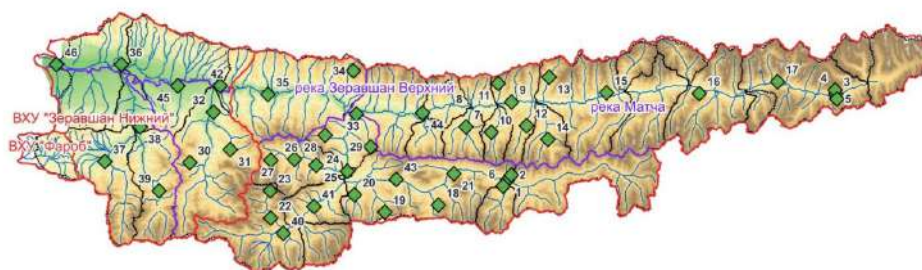
Figure 74. Distribution of potential sensor placement and sensor number in the Zarafshon River Basin. Red outlined regions indicate Water Management Areas (WMA) and purple regions indicate Water Objects (WOL). The colour gradient in the background displays elevation.
