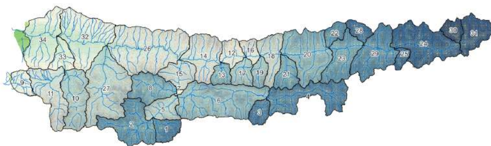
Figure 70. Sub-catchments in the ZRB in Tajikistan based on Strahler stream order number 7. The numbers indicate the sub-catchment number, the darkness of the blue color indicates its snow persistence, and thus indicates the importance of the sub-catchment to snow and glacier melt contributions to the river.
