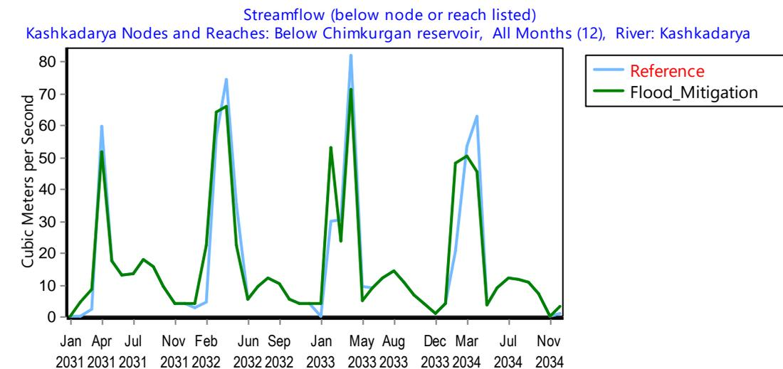
**Figure 48. Results for the Flood Mitigation scenario: streamflow below the Chimkurgan reservoir for the Reference and the Flood Mitigation scenario**
