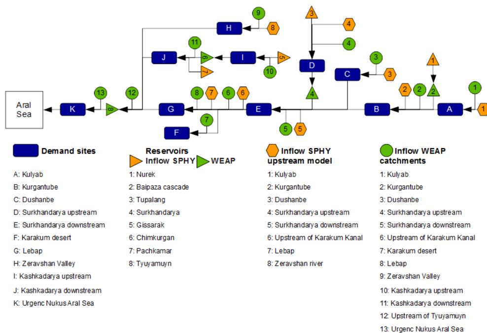
**Figure 42. The water resources system schematization for the Amu Darya river basin of the WEAP-Aral model**
