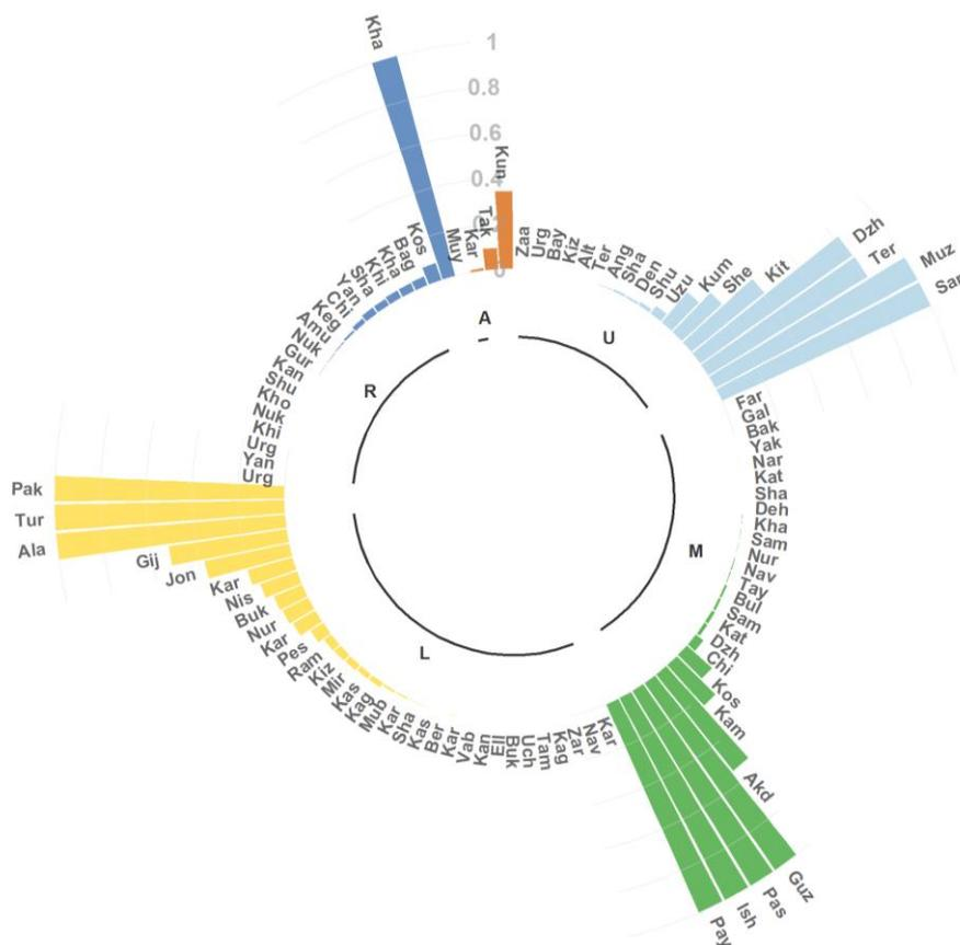
Figure 35. Flood risk radar plot ranking all districts in the five eco-hydrological zones (U=Upper, M=Mid, L=Lower, R=Riverine, A=Aral basin). Risk is scaled between 0-1 (low-high) and colors correspond to each ecozone. The 3 characters on top of the circular bar represent the first 3 letters of the district name.
