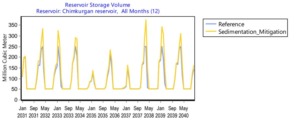
**Figure 46: Water stored in the Chimkurgan reservoir, with and without (Reference) sediment mitigation.**
