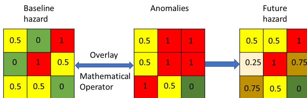
**Figure 4. Methodological framework to assess future hazards. The mathematical operator used in this project is 'addition'.**
