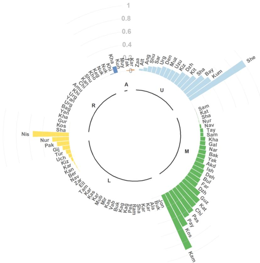
Figure 24. Landslide risk radar plot ranking all districts in the five eco-hydrological zones (U=Upper, M=Mid, L=Lower, R=Riverine, A=Aral basin). Risk is scaled between 0-1 (low-high) and colors correspond to each ecozone. The 3 characters on top of the circular bar represent the first 3 letters of the district name.
