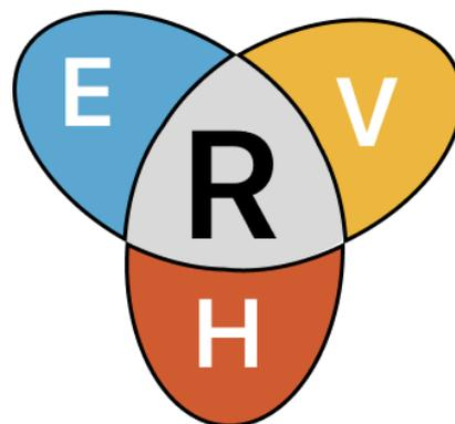
Figure 2. Risk (R) is defined as a function of Hazard (H), Exposure (E), and Vulnerability (V) components:
