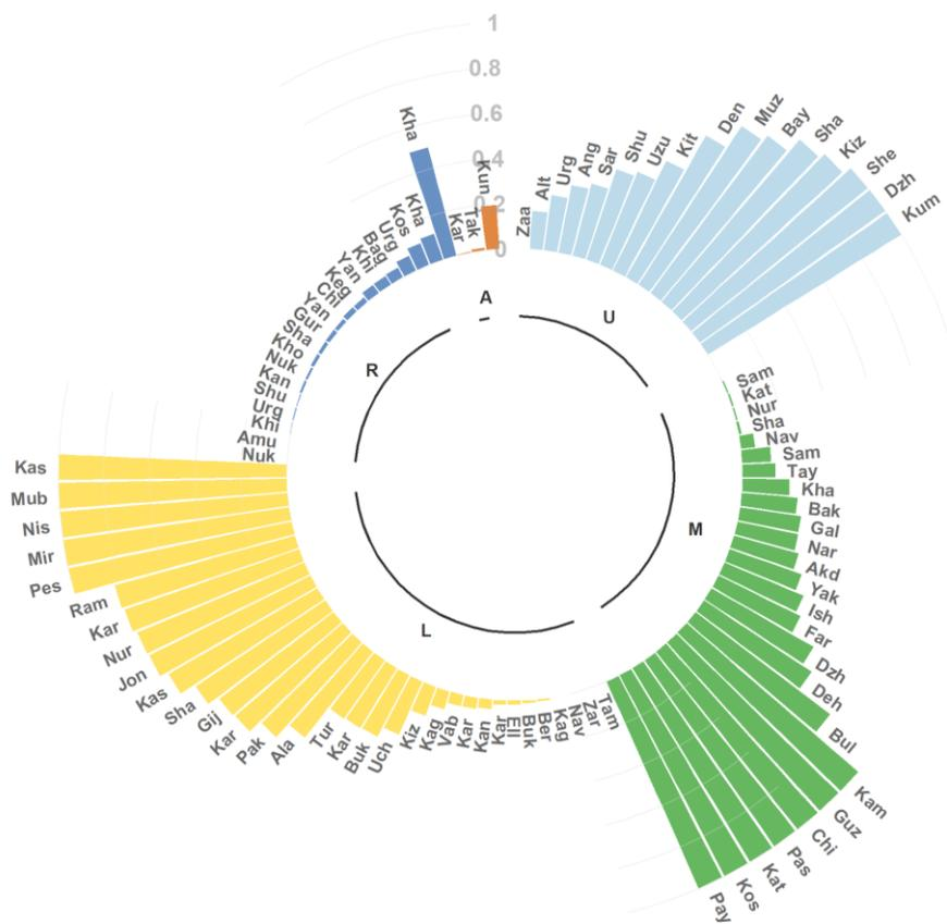
**Figure 28.** Erosion risk radar plot ranking all districts in the five eco-hydrological zones (U=Upper, M=Mid, L=Lower, R=Riverine, A=Aral basin). Risk is scaled between 0-1 (low-high) and colors correspond to each ecozone. The 3 characters on top of the circular bar represent the first 3 letters of the district name.
