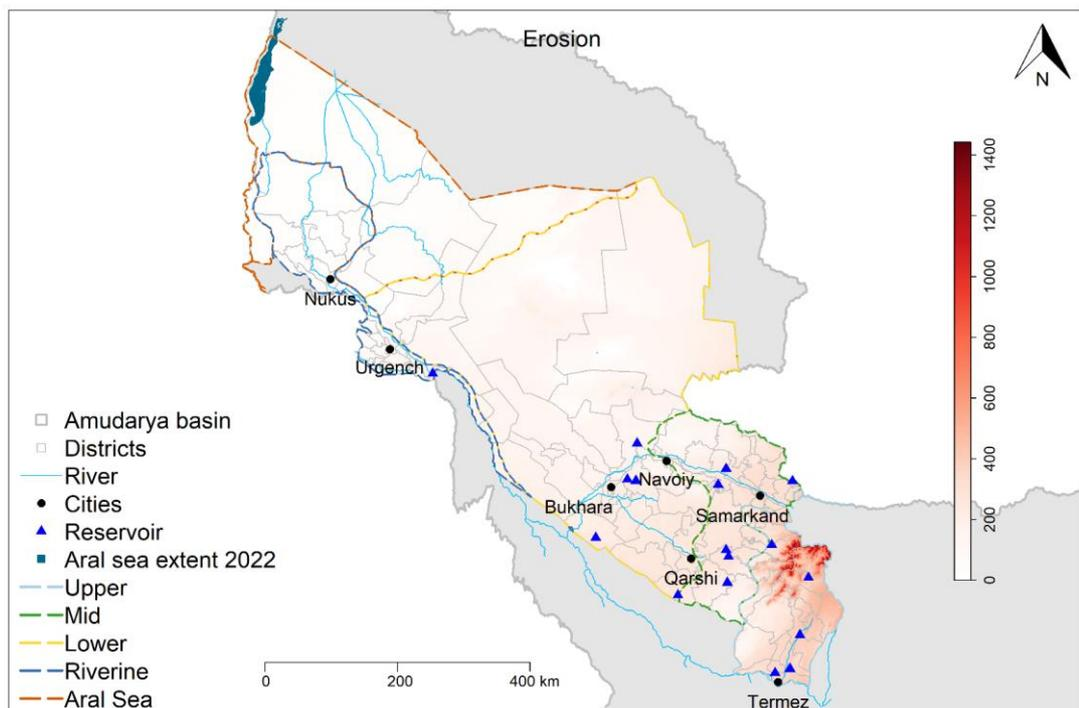
Figure 25. Baseline rainfall-induced erosion hazard map (in  $\text{MJ mm ha}^{-1} \text{h}^{-1} \text{yr}^{-1}$ ) for Amu Darya basin
