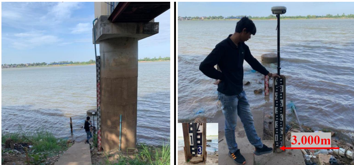
Figure 19: Surveyor was operating RTK rover to measure Neak Loeung gauge
