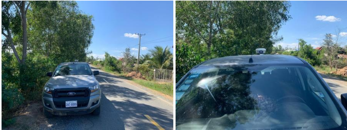
Figure 11: The photo of PPK rover was setup on the car
