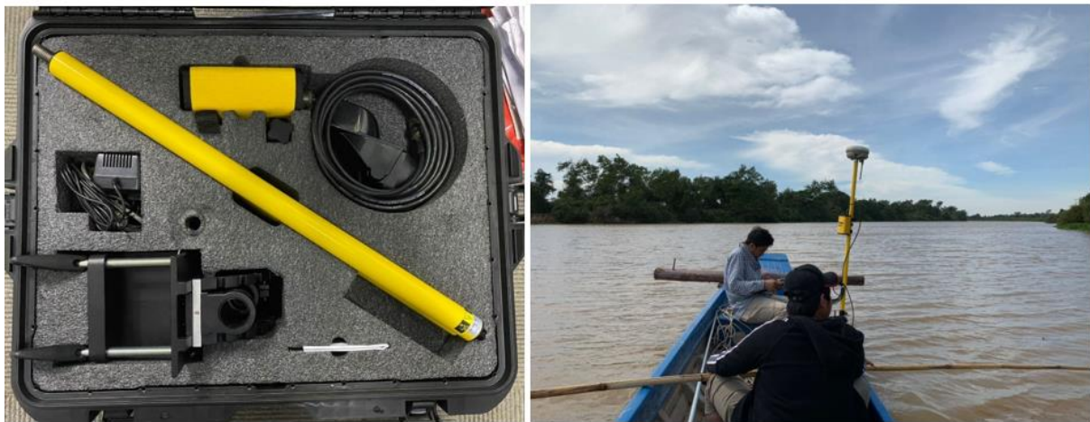
Figure 4: Surveyor was operating Eco-sounder on boat (right) and Eco-sounder system (left)
