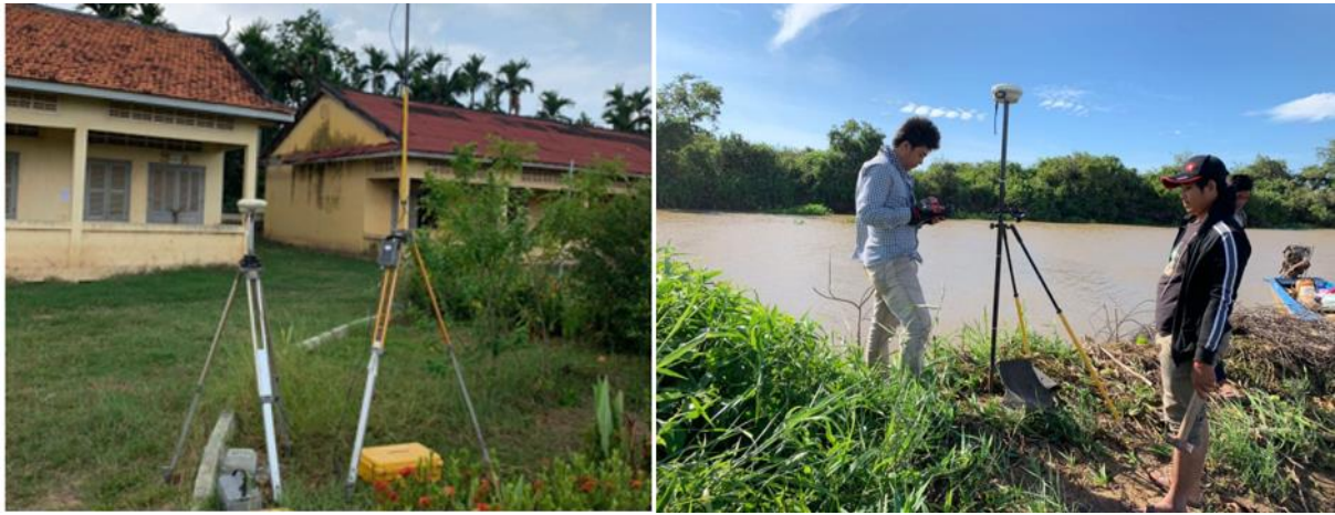
Figure 3: RTK Survey Base Station with Radio Link (left) and Rover (right)
