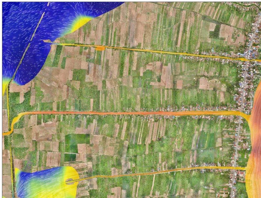
Figure 5-28 Localised Prek Cluster example model velocity output with particle tracing arrows.
