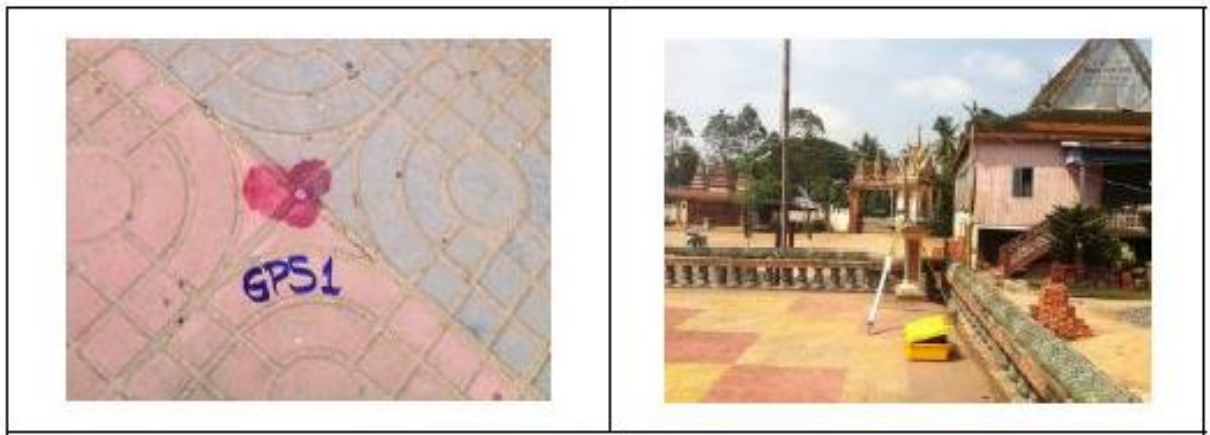
Figure 9: GPS Base Station GPS1 , vertical & horizontal national benchmark network
