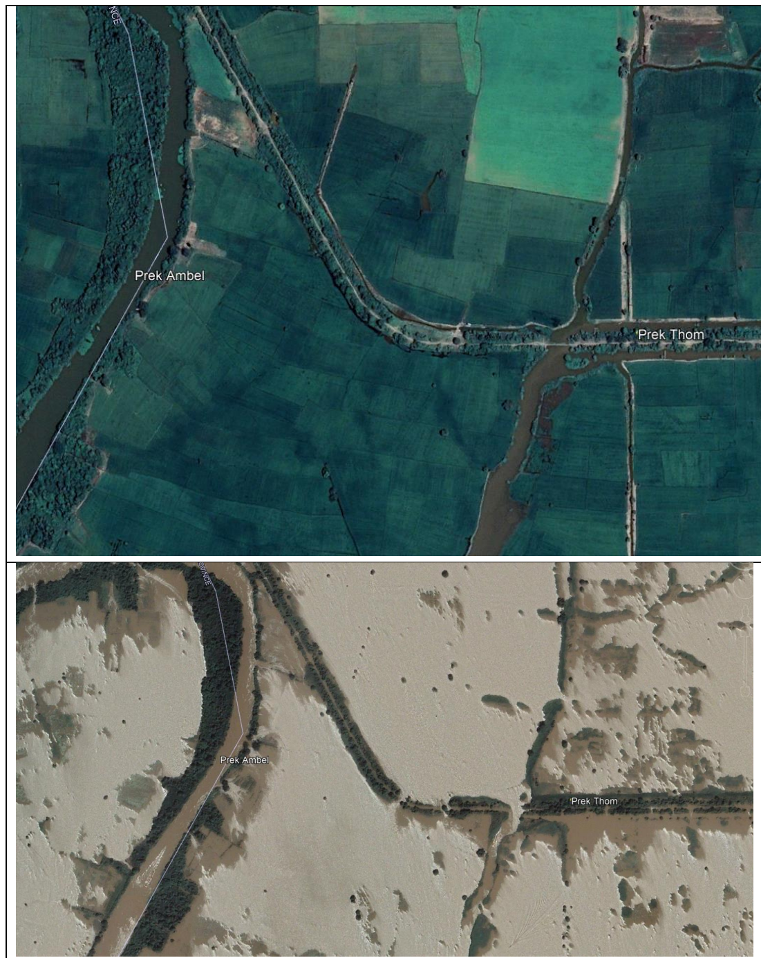
Figure 8-6 Prek Thom connection to Prek Ambel branch channel in dry and flood season (Source Google Earth Imagery 2019 and 2020 ). The direct connection to Prek Ambel is lost but the branch is wider than the main Prek channel
