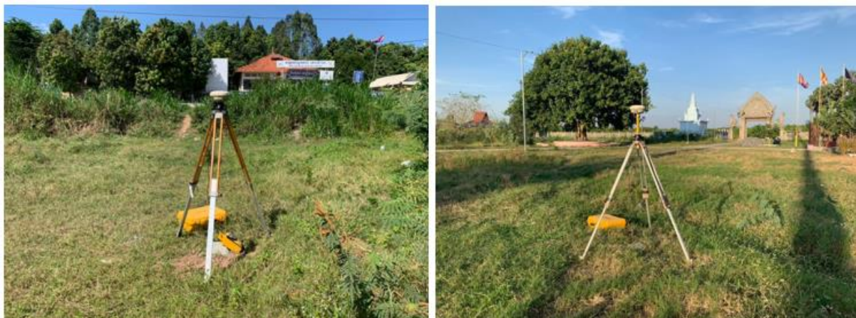
Figure 2: GPS Static Survey for Benchmark Control Points
