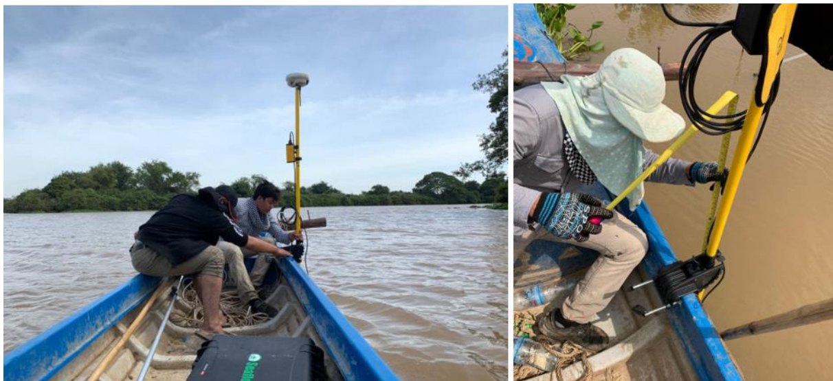
Figure 16: Surveyors operating Echo-sounder on boat (left) and surveyor checked water level and transducer height (right) before start survey
