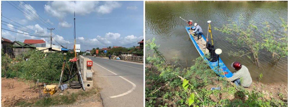
Figure 14: RTK base station with radio link (left) and surveyor was operating RTK rover on ground (right)
