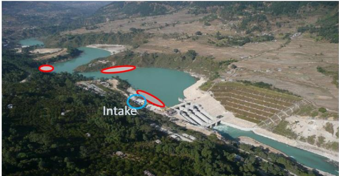
Figure 53. Areas of high sediment deposit upstream of the reservoir (red marked areas) and location of intake (blue marked area) (Source: NDRI, (2016))
