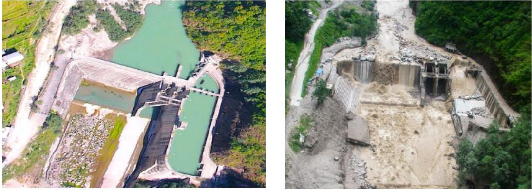
Figure 48. Damaged dam of the Upper Bhotekoshi Hydropower Project (45 MW) before (left) and after (right) flooding on 5 July 2016 on the Bhotekoshi River in Sindhupalchowk district, Nepal (Source: Bruen et al., (2017))
