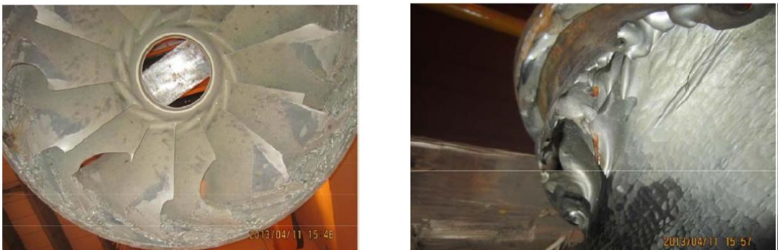
Figure 52. Photos of damage of runner and facing plates of Unit No: 2 of Kaligandaki 'A' hydropower (Source: Chhetry and Rana, (2015))
