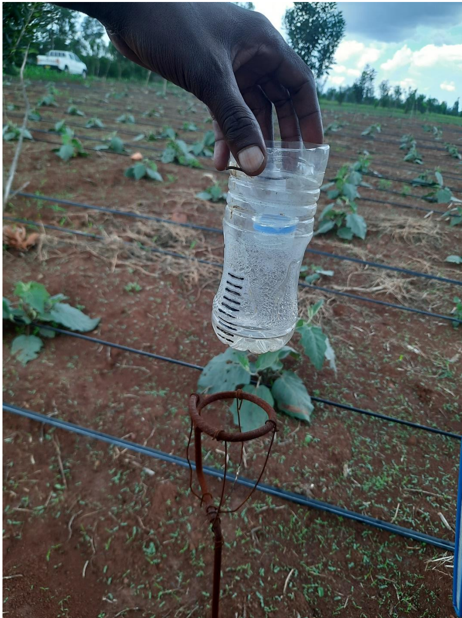
Rain meter made of water bottle for SOSIA calibration/evaluation.
