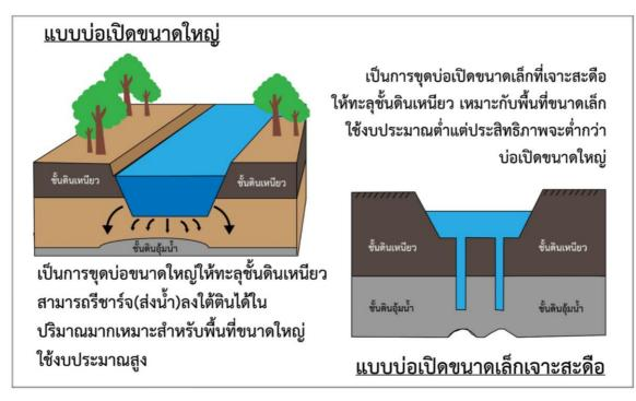
Figure 29: Concept of Open System Groundwater Bank (Large and Small) Source: American Groundwater Solutions
