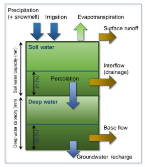
Figure 2. Schematic overview of the core processes in the WEAP catchments' calculations.
