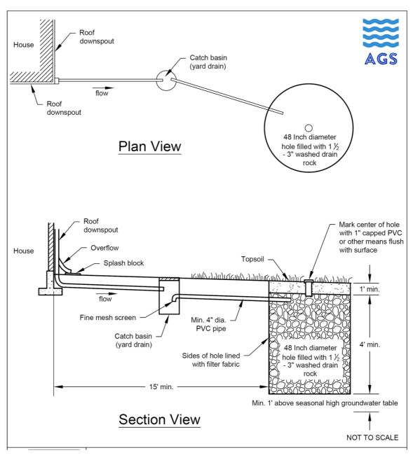
Figure 30: Typical Plan and drawings for Dry Well Construction (Closed System) Source: American Groundwater Solutions
