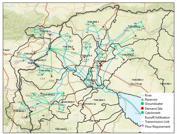
Figure 3. Schematization of the WEAP model for Oddar Meanchey and Banteay Meanchey.
