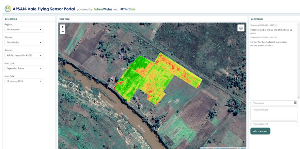
Figure 19 Screenshot of the APSAN-Vale Flying Sensor Portal, showing the option to select a map on the left side, the vegetation status map in de middle and some example comments in the right section
