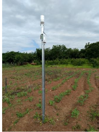
Figure 8 The TAHMO station in the measurement field.
