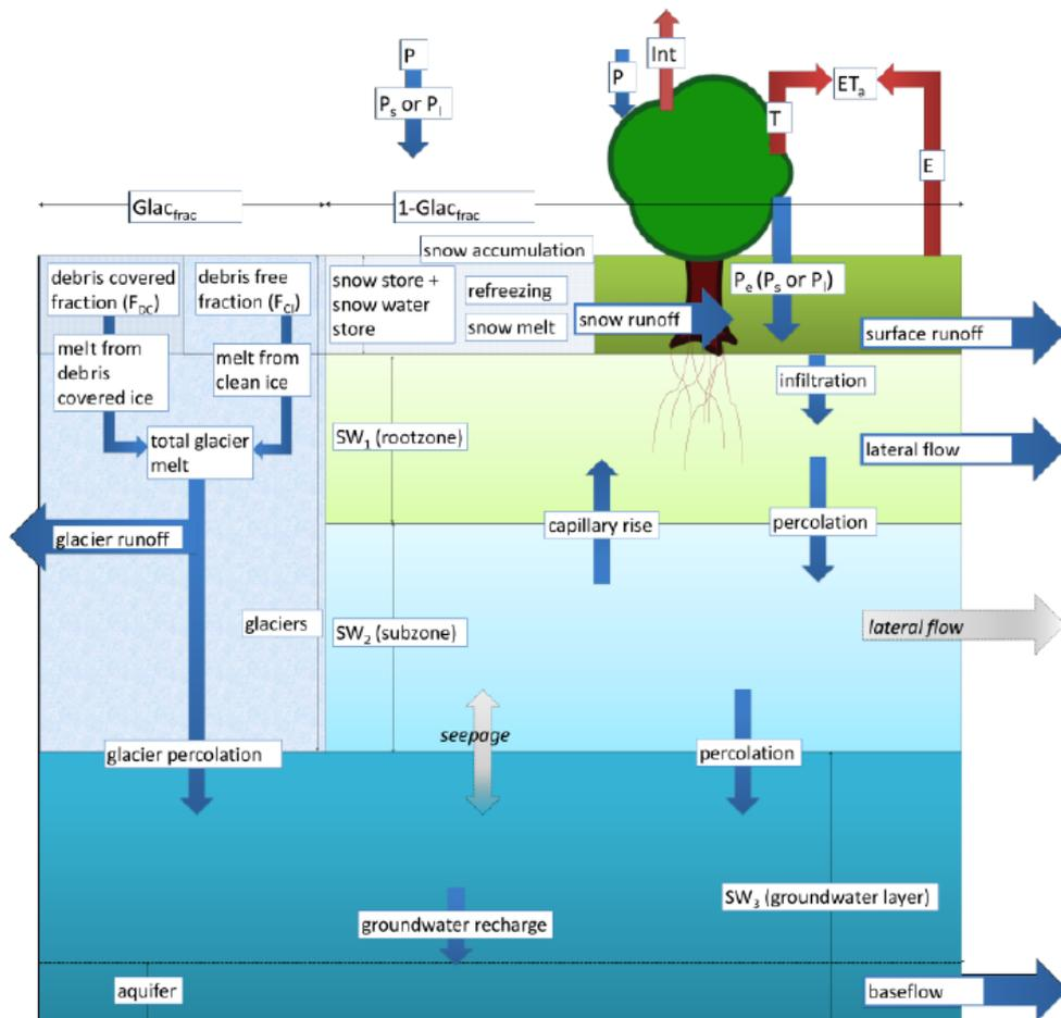
Figure 2-2: Conceptual scheme of the hydrological model SPHY
