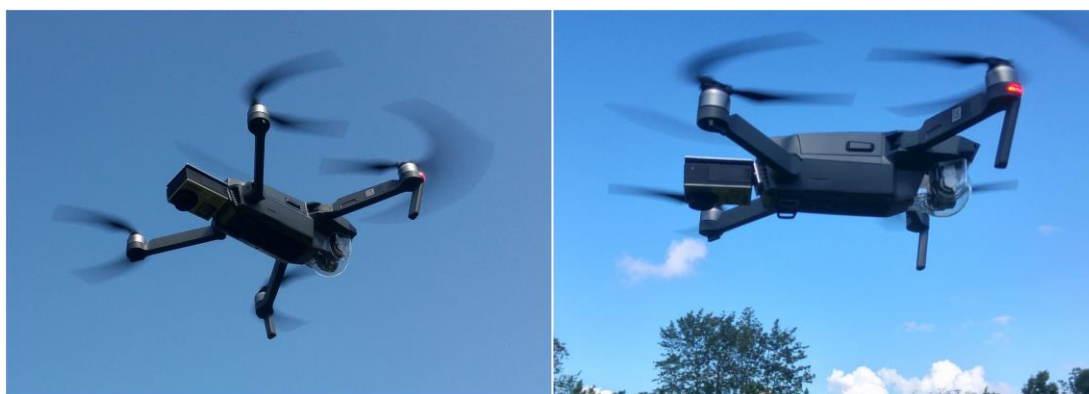
Figure 7. ThirdEye's modified flying sensors, with a NIR Go Pro camera mounted on the back of the flying sensor.
