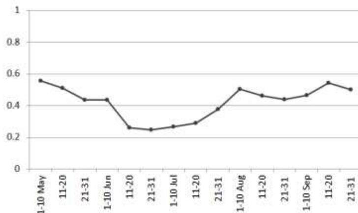
**Figure 10. Graph showing a typical Landsat-based NDVI curve extracted for a cropland in the period May to September in Huambo province. The end of May shows decreasing NDVI values associated with the end of the production period. The NDVI curve then increases from mid-July which is associated with the start of the next growing season.**
