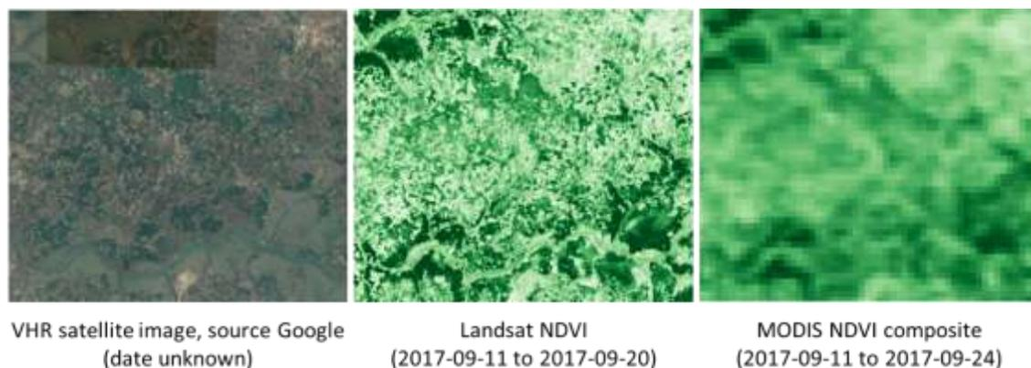
**Figure 4. Examples of Landsat and MODIS based NDVI for a subset of the area covered by Landsat. The Landsat and MODIS based NDVI data is shown using the same legend where darker shades of green represent higher NDVI values. For context, the very high resolution image on the left was obtained from Google.**
