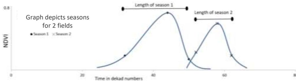
**Figure 5 Graph showing how the start and end of a growing season can be determined from an NDVI time series. This example shows the NDVI curves for 2 separate fields, containing a crop in season 1 and in season 2 respectively.**
