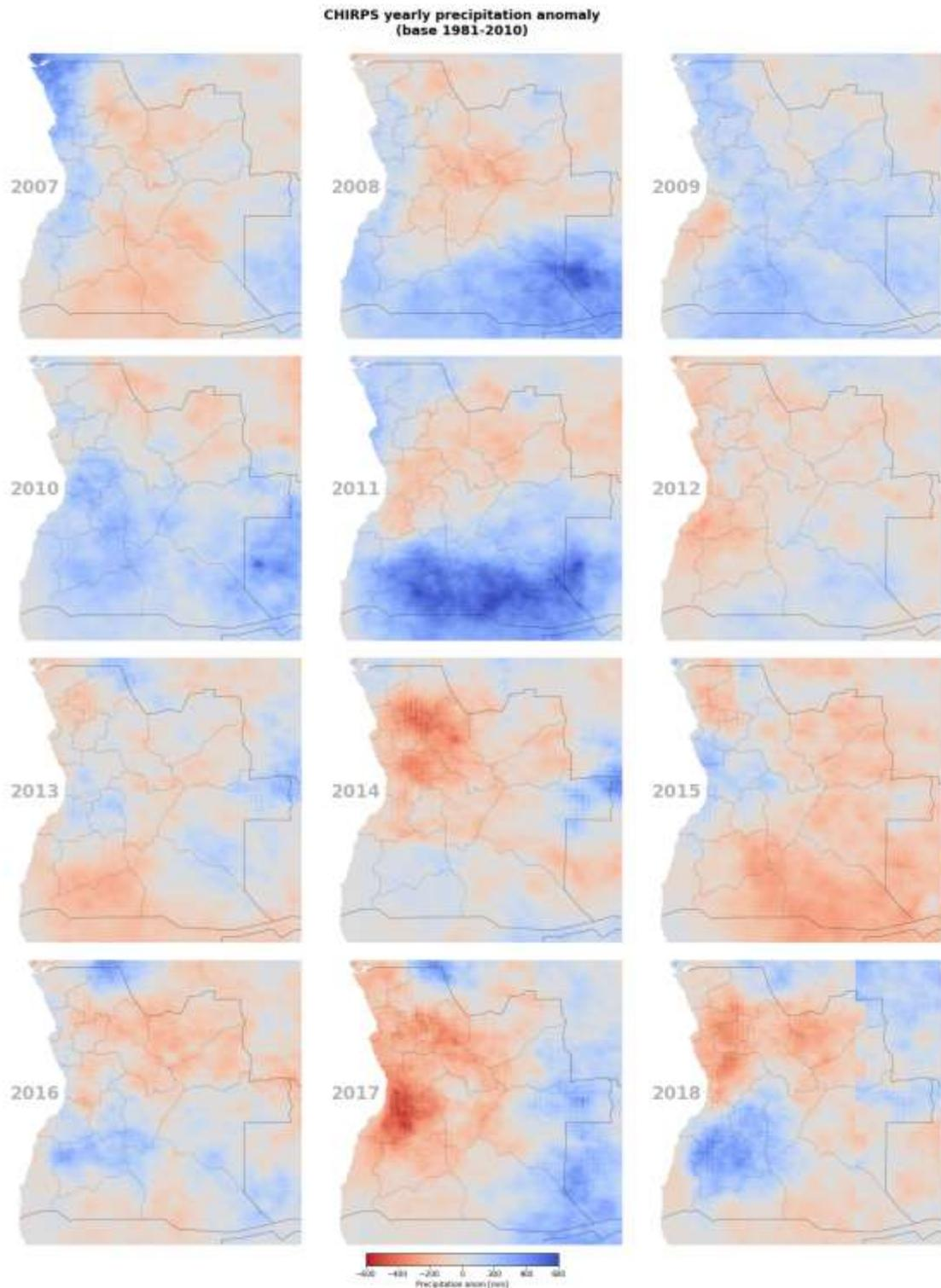
**Figure 12. Maps showing annual precipitation anomalies for 2007 to 2018 based on CHIRPS rainfall data<sup>1</sup>. Red areas have received significantly less rainfall than normal, whilst blue indicates significantly lower annual rainfall than normal (where ‘normal’ refers to the base period 1981-2010). A figure showing annual rainfall anomalies from 1981 to 2018 is included for additional information in Appendix 1.**
