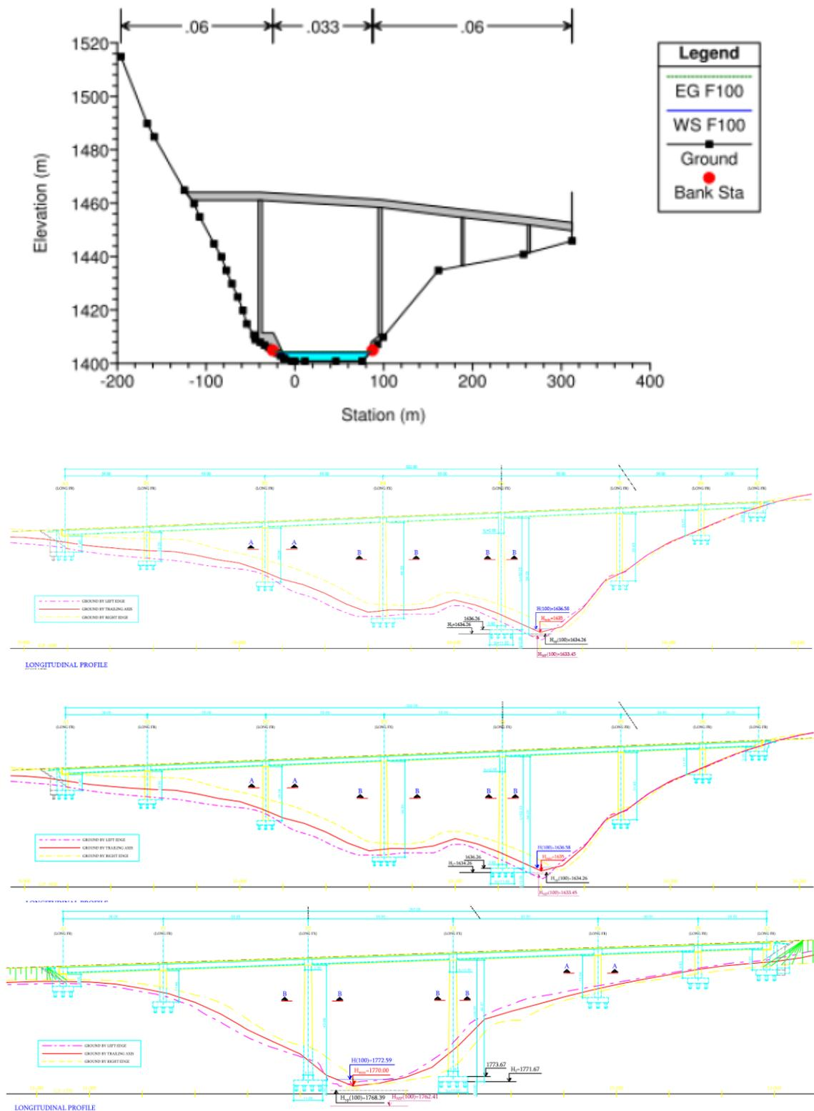
Figure 22: Drawings of bridges designed for the project, indicating high elevation difference between road surface and water level (IDOM, 2018a).
