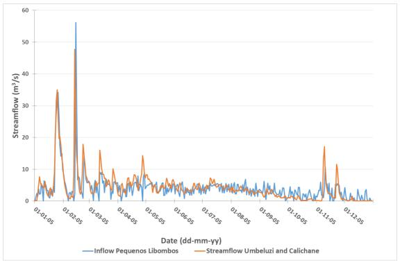
Figure 35. Comparison of inflow into Pequenos Libombos and streamflow of Umbeluzi and Calichane for 2005.
