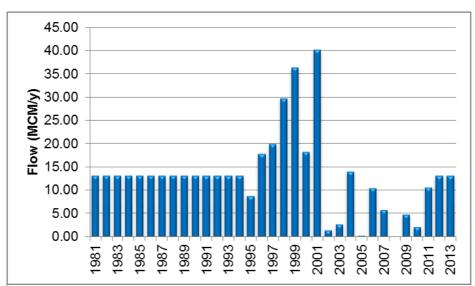
Figure 33. Total yearly streamflow for Calichane from 1981-2013 measured at gauging station E-0019H.
