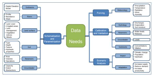
Figure 26. Overview of data needs to build water allocation models.
