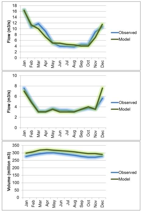
Figure 10. Observed and modelled inflow into Pequenos Libombos (top), outflow from Pequenos Libombos (middle), and volume of Pequenos Libombos (bottom).
