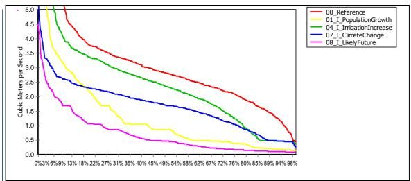
Figure 20. Annual Umbeluzi streamflow at outlet point into Indian Ocean (top) and exceedance probability of Umbeluzi streamflow at outlet (bottom), expressed as % of months, for the Impact Scenarios.
