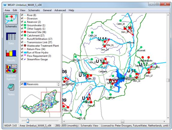
Figure 6. Screenshot of WEAP: GIS interface to develop the schematization.
