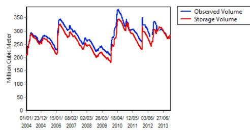
Figure 37. Observed reservoir volume (blue line) and simulated reservoir volume of the uncalibrated model (red line) from 2004 to 2013.
