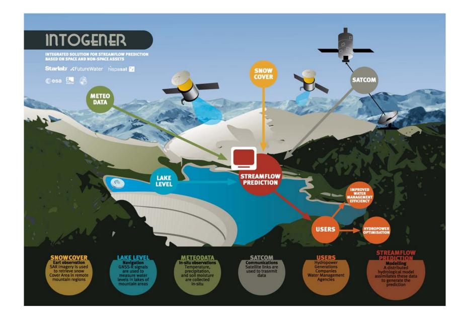
**All the information** (from in situ instruments, satellite observations, historical data, and model output) is centralized on a **secure server** running a database as well as services required for data flow and automation.
