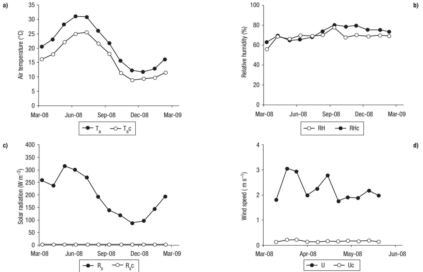
**Figure 4.** Comparison of the meteorological variables measured below the cover and 2 m aboveground. Monthly values of a) air temperature ( $T_a$  and  $T_{aC}$ ), b) relative humidity (RH and RH<sub>C</sub>), c) solar radiation ( $R_s$  and  $R_{sC}$ ), and d) weekly values of wind speed ( $U$  and  $U_C$ ).
