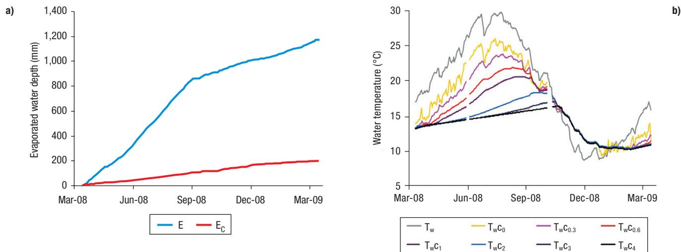
**Figure 3.** Annual evolution of (a) evaporated water depth and (b) water temperature profile for covered and uncovered conditions.  $E$  and  $E_c$  are the evaporation rate for uncovered and covered conditions respectively.  $T_w$  is the water temperature for uncovered conditions and  $T_{wC_i}$  are the water temperature for covered conditions at the depth  $i$  (m).
