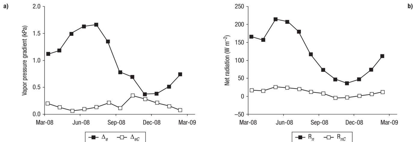
**Figure 5.** Annual evolution of monthly averages of (a) evaporation driving force for open-water ( $\Delta_e$ ) and shaded conditions ( $\Delta_{eC}$ ), and (b) modelled open-water net radiation ( $R_n$ ) and measured net radiation under the cover ( $R_{nC}$ ).
