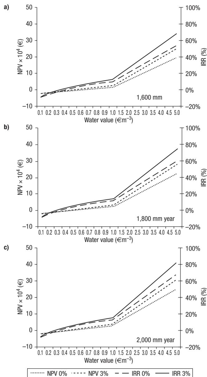
**Figure 8.** Net present value (NPV) and internal return rate (IRR) for three levels of Class-A evaporation rate: a) 1,600 mm year<sup>-1</sup>, b) 1,800 mm year<sup>-1</sup> and c) 2,000 mm year<sup>-1</sup>. Filter cleaning requirements are 0 and 3%. Water values range from €0.1 to 5 m<sup>-3</sup>.
