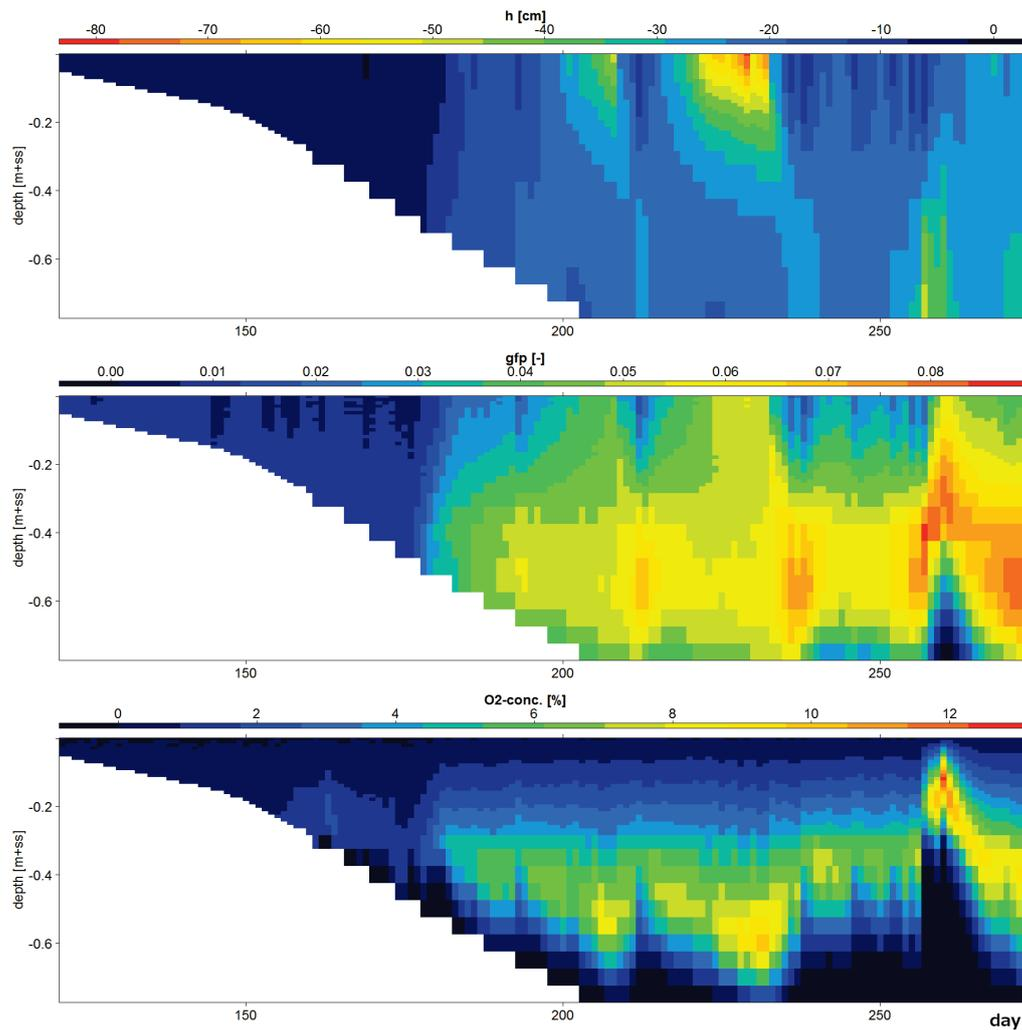
Figure 9: Differences of soil water pressure head ( $h$ ), gas filled porosity ( $gfp$ ) and oxygen concentration ( $O_2$ -conc) in the root zone for the growing season of 1998, for simulations with a fixed and with a dynamic crest (Figure 8). Given values = results dynamic crest - results fixed crest. The root depth increases during the growing season, with a maximum depth of -0.7m+s.s. around day 200; this explains the white area in the figures.
