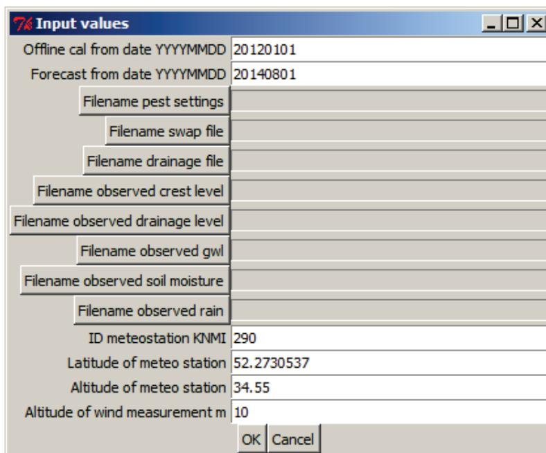
Figure 16: Start screen for the optimization tool, where input values and files should be provided.
