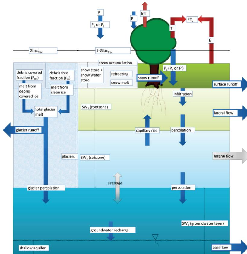
Figure 6: SPHY model concept. Several of these concepts, such as the glacio-hydrological module of the model, are optional and switched off in the current application ([www.sphy.nl](http://www.sphy.nl)).
