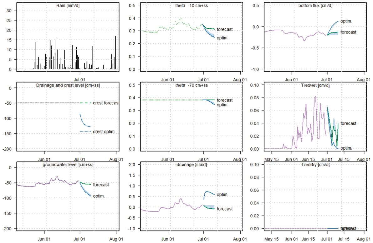
Figure 20: Example of forecast and optimization of the crest level for wet conditions. In order to limit future oxygen stress (Tredwet, forecast), the crest level needs to be lowered (crest optim., see also Figure 18). This will increase the drainage flux, lower the groundwater level and soil moisture contents (theta), and limit Tredwet..
